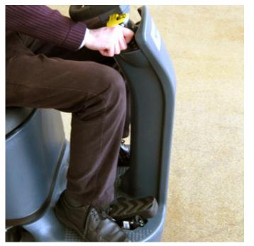
**3** Turn the ignition key to "0", then try to start the machine without pressing the pedal speed.
