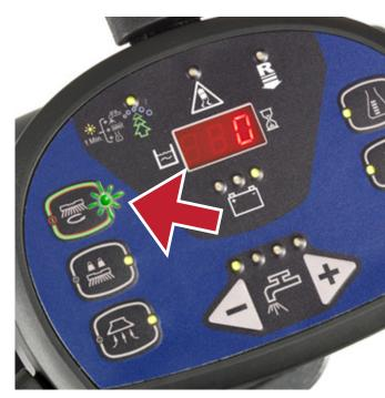
Check if the green switch Led is flashing. Wait until the light is steady.
