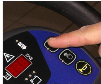
8. Press the detergent flow control switch. The number of display shows the detergent concentration level in the solution.
