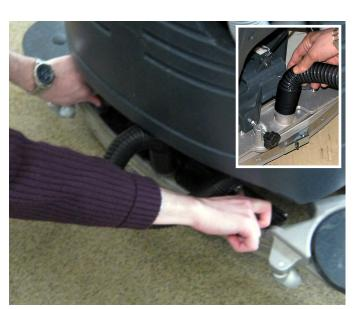
4. Install the squeegee and fasten it with the handwheels, then connect the vacuum hose to the squeegee.
