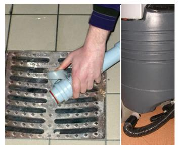
12. At the end of the work. Empty the recovery tank with the hose. Then empty the solution tank by opening the left drain tap and using the adapter and the vacuum system hose.
