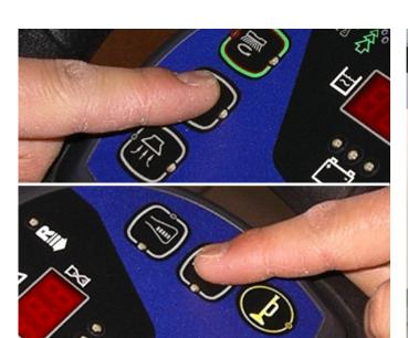
function switch. If necessary press the mute functionswitch for reduce the noise.
