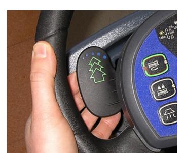
9. Lift the EcoFlex<sup>™</sup> lever whenever you temporarily need a greater cleaning power.
