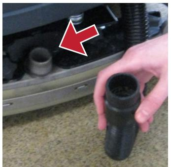
**1** Check if the suction hose is correctly mounted and cleaned.
