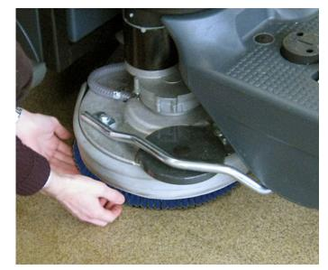
5. Place the brushes or the pad-holders under the deck. Use the appropriate brushes to clean the floor.
