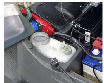
3. Fill the EcoFlex tank with a detergent suitable for the work to be performed (highly concentrated detergent).
