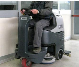
10. If necessary press the extra pressure 11. Push the pedal speed for starting floor cleaning. If solution applied flows outside the brush housing during use, reduce the flow of solution. Switch off the machine using the key.
