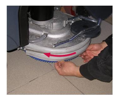
15. Remove the brush by turning as indicated with the figure and clean them.
