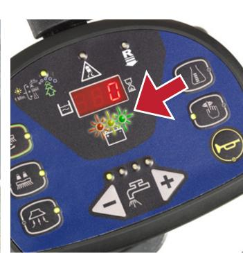
2 Check if there isn't any brush motor 3 overload i.e. 3 battery Ledsflash simultaneously.
