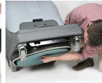
4. Rotate the retainer and remove it from the machine.
