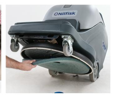
5. Remove the pad and check the status. If needed, change it. Be sure to use correct burnishing pad depending on floor type and application
