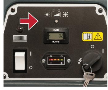
1. If the battery is on charge, check if the battery charger indicator shows a green light (it means the battery is fully charged)
