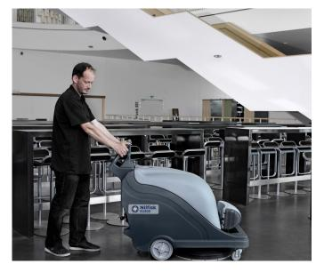
11. Press switches on the handle to activate pad rotation and start burnishing, remember to always keep the machine moving. Too long time on the same surface can damage the floor
