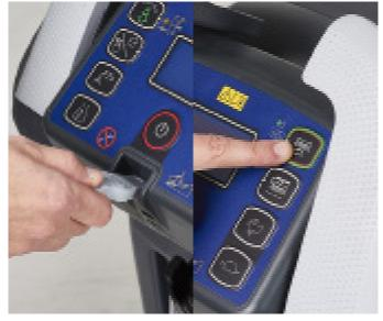
6. Insert the operator key, then start the machine by pressing the One-Touch button. To engage the brush, slightly press the drive paddle and then release it.
