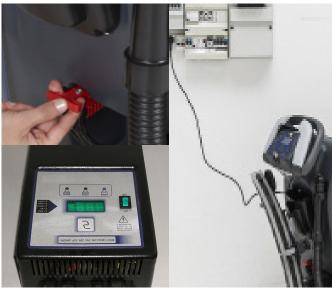
19. Charge the batteries: Connect the battery charger cable to the electrical socket.
