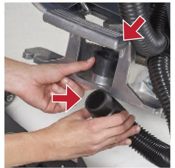
Check if the suction hose is correctly installed and cleaned.
