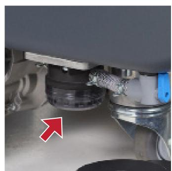
Check if the solution filter is cleaned.
