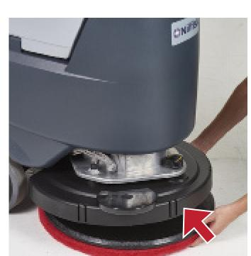
Check if the brush are correctly installed and not worn out or if there are external materials avoiding brush rotating.
