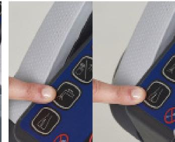
9. To change the solution flow level push the solution button and change flow level according to the cleaning performance and application.
