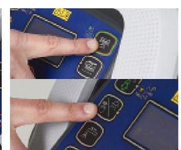
If necessary press the extra pressure function (hold for one second).
