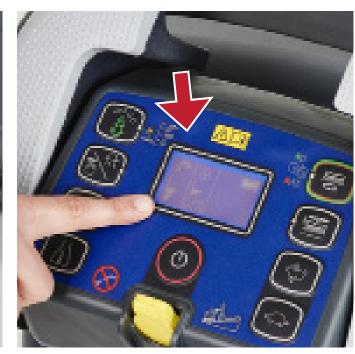
2 Check if there isn't any brush motor 3 overload "WARNING ALARM F2" on the display.
