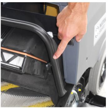
3. Check if the gasket is damaged.
