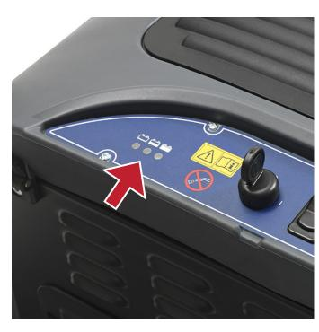
1. Check if the battery is charged and that the charger cable is disconnected from the main.
