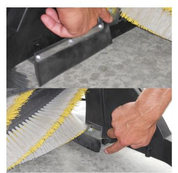
1. Check if the flaps are correctly adjusted and not worn out.
