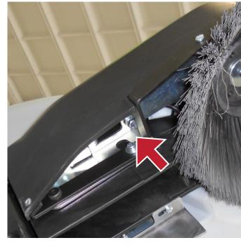
2 Adjust the side brooms position by the register screw.
