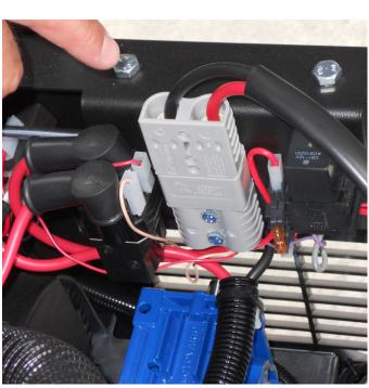
2. Check if the main battery connector is properly connected.
