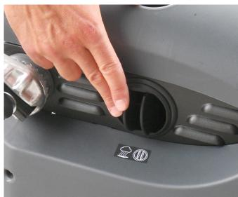
the "wet by-pass" port to avoid damaging the dust filter. Close the "wet by-pass" port to restore proper vacuuming.
