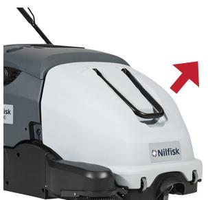
handle and drive it to the area of disposal and empty it and put the hopper back on the machine
