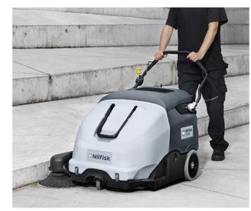
6. Drive the machine straight forward. Adjuting speed depending working conditions/quantity of debris.
